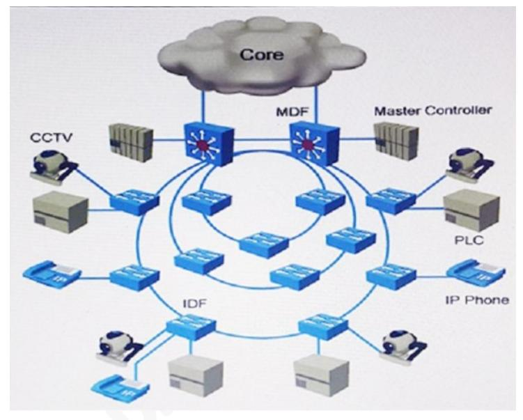
Refer to the exhibit. This smart city has decided to deploy a converged network for video surveillance and applications for utility services. These new applications are delay-sensitive and require strict convergence times of less than 50 milliseconds. The network is expected to have up to 50 intermediate distribution frames per ring. Which protocol provides less than 50 milliseconds convergence?
