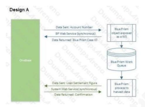
Here a Blue Prism object is exposed as a web service. OneBase calls this service providing the account number. The Blue Prism object add the case to a work queue and then returns the Case ID to complete the web service call.
