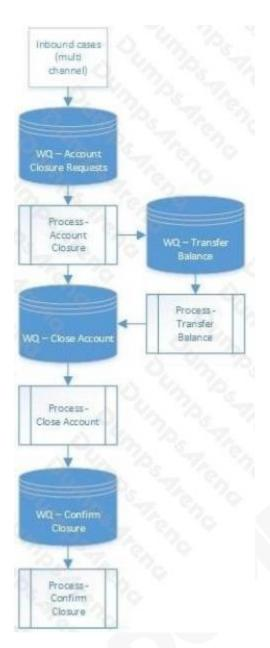
Cases come into the Account Closures Work Queue and are processed by the Account Closure process which determines if they are "Nil Balance" or "Balance to Transfer" scenarios. Before adding the case to the relevant work queue, a check is made to see if an identical key has been added to the work queue today. If so the case is not added.
